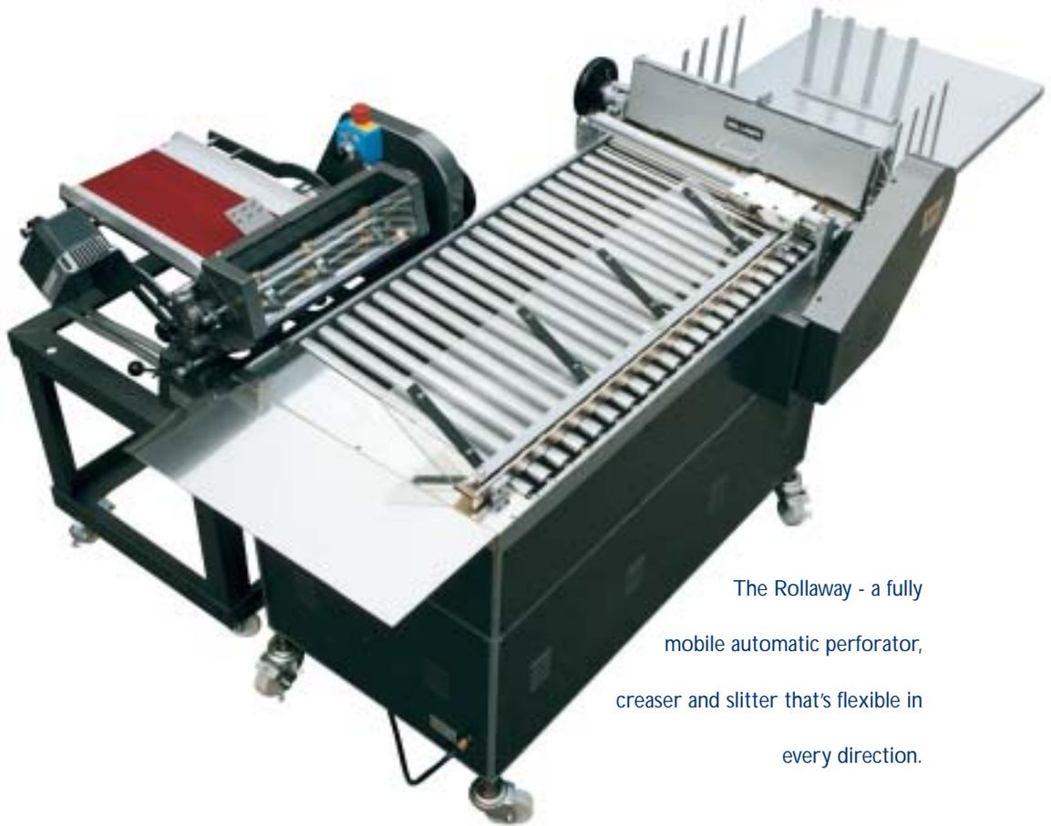
The Rollaway - a fully mobile automatic perforator, creaser and slitter that's flexible in every direction.
