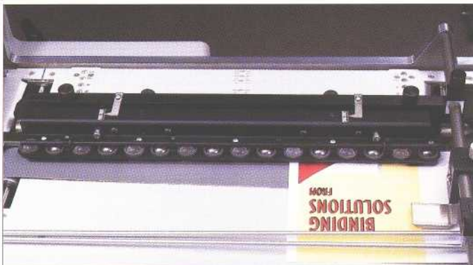
Side lay register table ensures that the paper is correctly aligned before feeding into the rollers.
