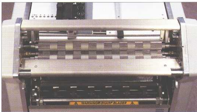
Combination fold rollers grip the paper positively to eliminate any possibility of paper slippage.
