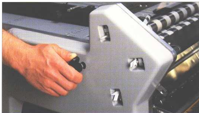
Fold roller pressure settings give completely accurate pressure on each fold roller and no marking.
