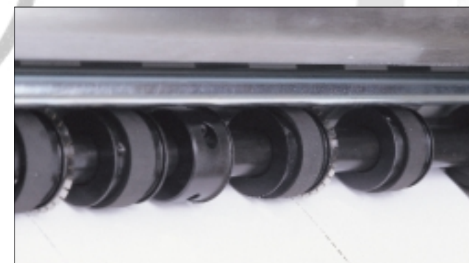
UFO perforating/scoring unit is standard equipment on the UFO 1 and an option on UFO 2/2B.
