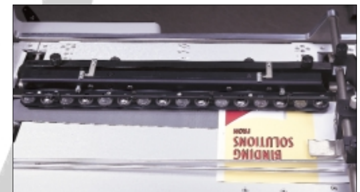
Side lay register table ensures that the paper is correctly aligned before feeding into the rollers.
