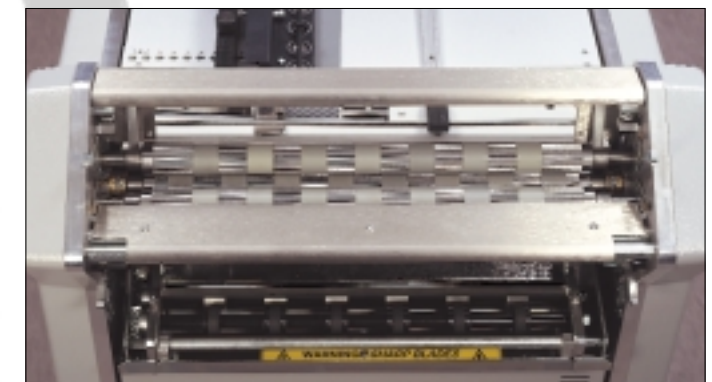
Combination fold rollers grip the paper positively to eliminate any possibility of paper slippage.
