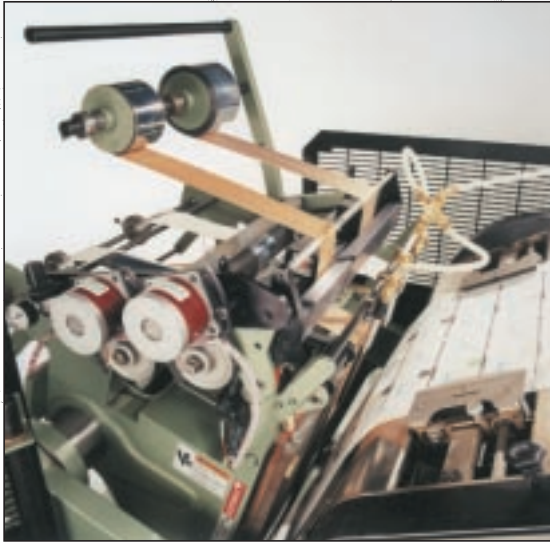
▲ Close-up of electronic leafer and honeycomb toggle base.
